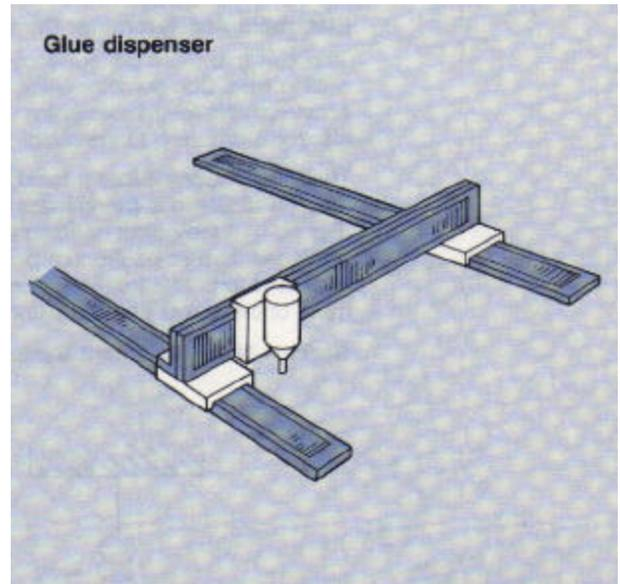
A simple X-Y positioning system is constructed as a gantry with three linear motors. The X-Y motion is controlled with two SI indexers/drivers. For the parallel X axes one SI pulse/direction is used to synchronize it with the linear motor and drive.
